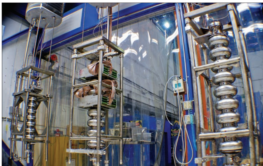
Three electropolished cavities await cryogenic testing at Jefferson Lab: an AES cavity (right); a large-crystal niobium cavity, built in-house, with T-mapping system mounted (middle); and a prototype cavity for the facility's CEBAF upgrade (left) processed using the "ILC recipe". (Courtesy Jefferson Lab.)
